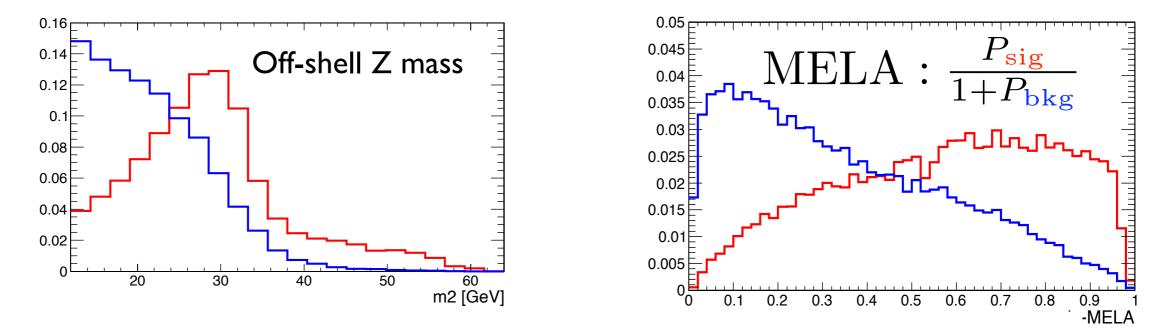
A toy study using CMS-like analysis shows that using MELA increases the search sensitivity by ~15-30% compared to using only the 4I mass
