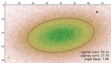
The solid lines correspond to a 2-d Gaussian fit. Axis units are pixels.
