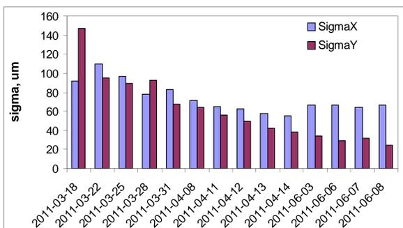
Beam size evolution from Marc – June 2011. Note that the days are not equispaced.
