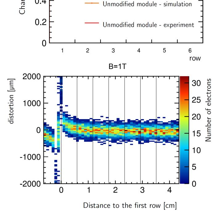
Without magnetic field the electrons follow the electric field lines and end up in the gap between modules. With the introduction of a magnetic field ExB effects change the electron drift path resulting in a distortion of the electron arrival positions near the module border.
