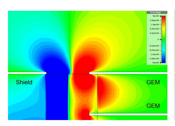
The addition of a field shaping wire reduces the field distortions. The charge collection efficiency could be improved by 30% both in simulation as well as in the measurement.
