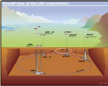
ALICE is located underground with 30 m of overburden rock. Only atmospheric muons with energy  $E_\mu > 15$  GeV can reach the experiment.
