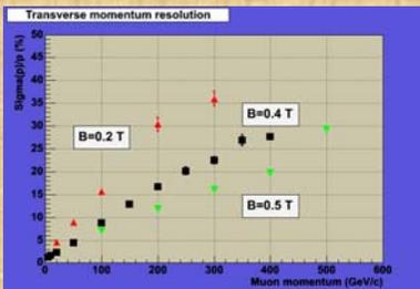
The momentum resolution of the muons improves with the magnetic field strength  $B$  in the central detectors. At  $B = 0.5$  T  $\Delta p/p = 30\%$  for  $p_\mu = 500$  GeV/c.
