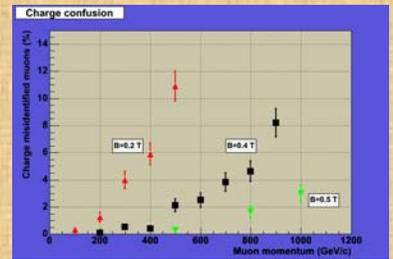
Muon charge sign misidentification for different values of the magnetic field  $B$ .
