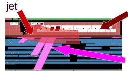
energy deposits in TileCal cells fraction of red area indicates the amount of energy in the cell
