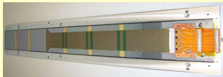
o Front-end chip of LHCb Vertex, trigger tracker, silicon tracker and pileup detectors.
