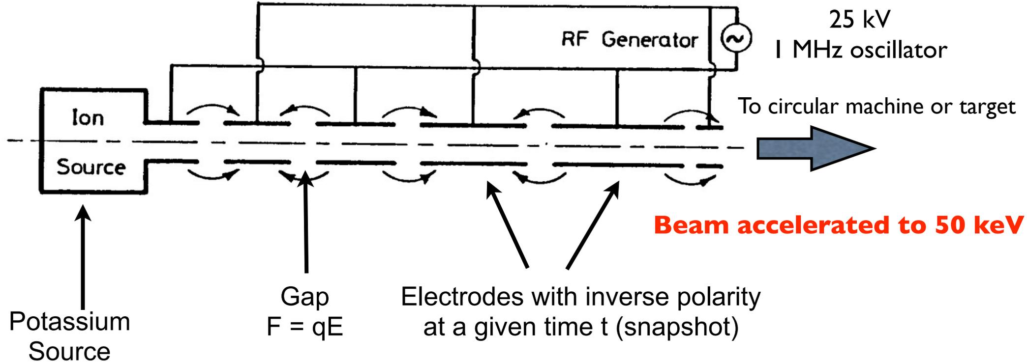
First linac composed by drift tubes interleaved by acceleration gaps powered by an RF generator. (1928)
