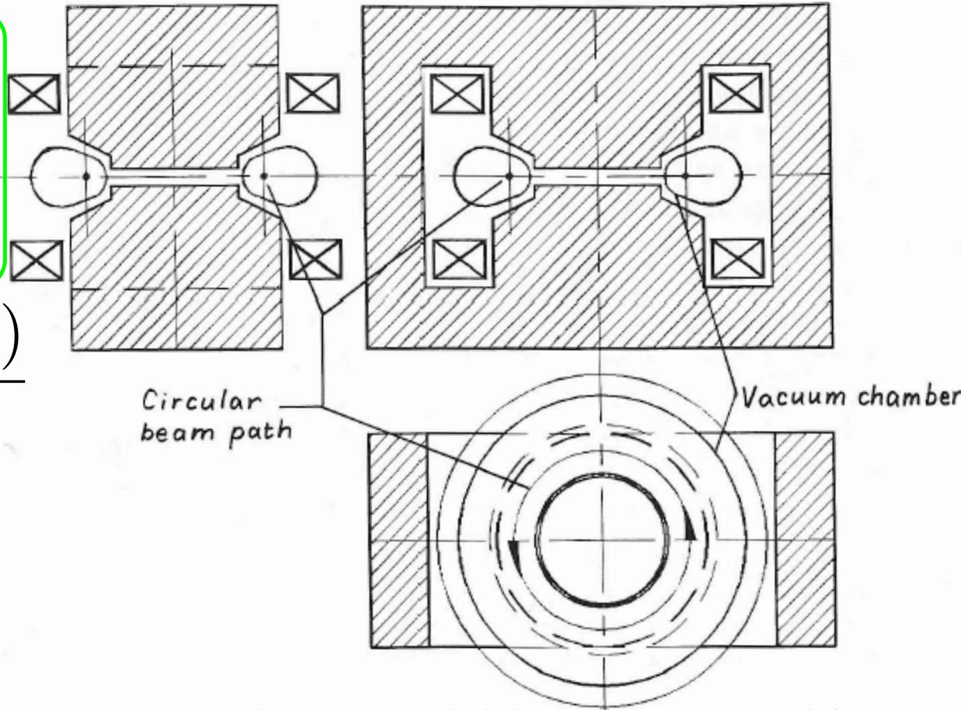
Kerst built the first one in 1940 for electrons up to 2.3 MeV
