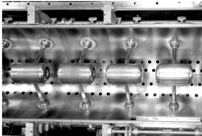
Inner structure of Linac I (Alvarez type). The drift tubes are supported on stems, through which the current for the quadrupole magnets (located inside the tubes) and the cooling water are supplied.
