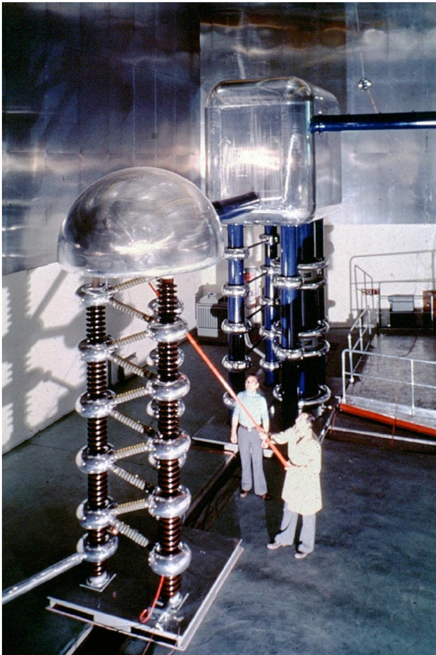
High voltage unit composed by a multiple rectifier system
