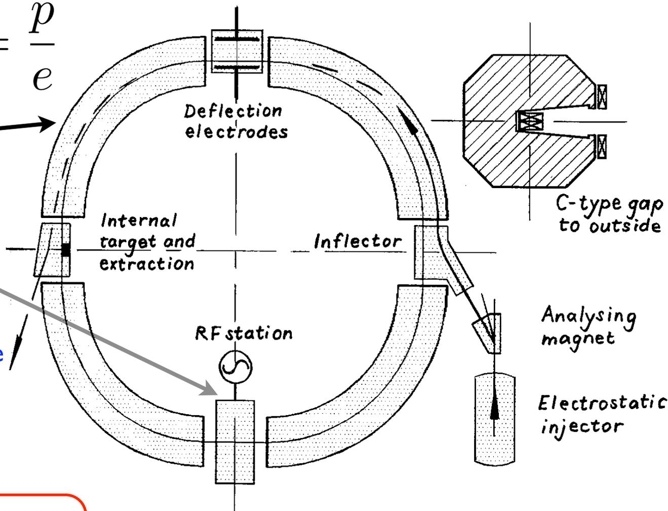
Weak focusing machine: no quadrupoles yet
