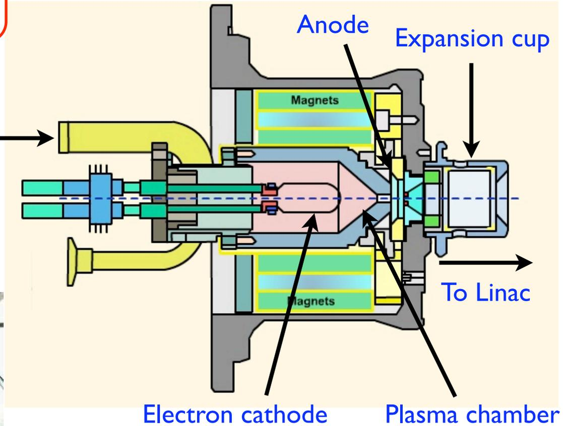
Proton exiting from the about 1 mm<sup>2</sup> hole have a speed of 1.4 % c,  $v \approx 4000$  km/s
