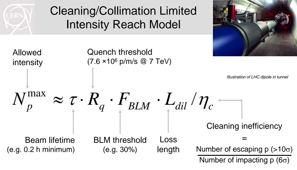
Collimation performance can limit the intensity and therefore LHC luminosity.
