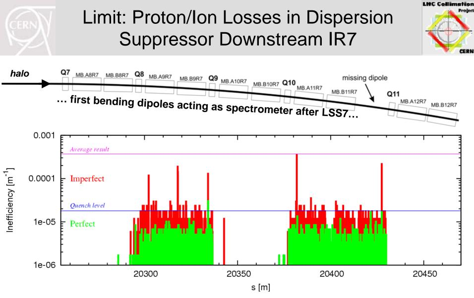
Collisions p on carbon generate off-momentum protons (mostly single-diffractive scattering). Are kicked out by the first bending dipoles (classical spectrometer).
