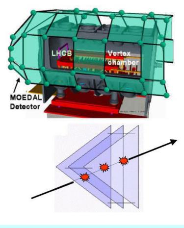
Remove the sheets after some running time and inspect for 'holes'
