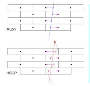
Derive the Time-of-flight from hit pattern in the muon chambers  $\Rightarrow$  Measure  $\beta$  of the particle from the time-of-flight!!
