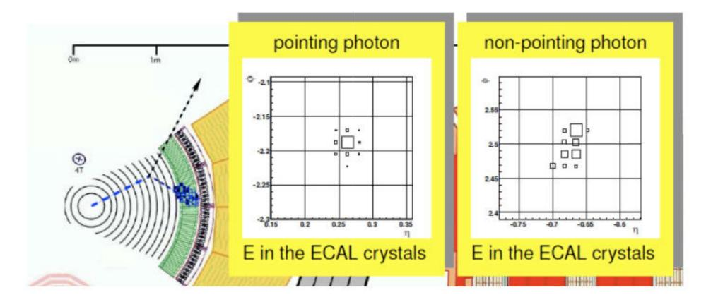
Possible both in CMS and ATLAS from the shower shape in the electromagnetic calorimeters. Example: CMS projective crystal calorimeter
