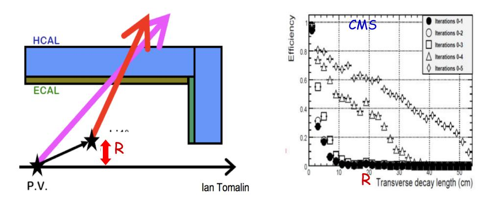
High efficiency possible for charged particles (max R ~ 50 cm)...
