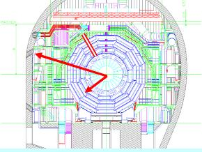
Sparticles stopped in the detector,walls of the cavern, or dense 'stopper' detector. They decay after hours---months...
