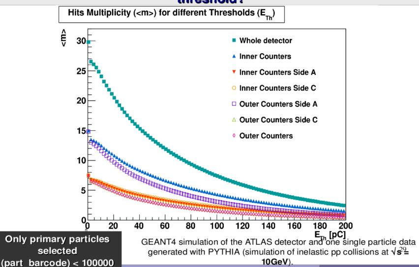
Smooth behaviour of multiplicity as a function of pulse height threshold. Detector is not fully saturated. Can be used to estimated luminosity.
