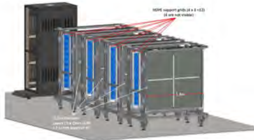
Figure 3: The basic structures of the MAPP-mQP without the outer VETO layer, the support structures emphasized.
