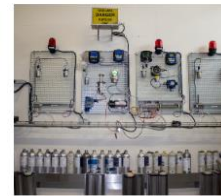
The test platform for detecting gas (including ODH). The bottles at the bottom of the image contain different types of gas used for tests.
