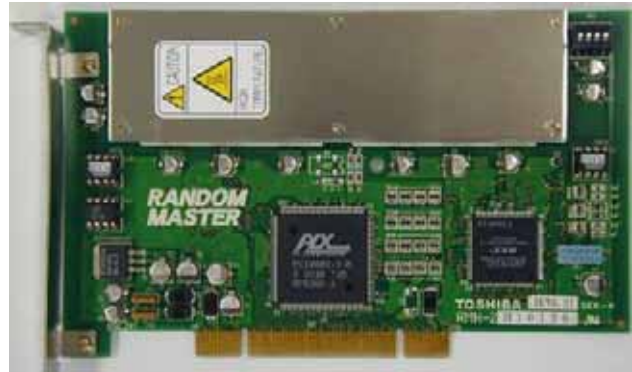
Figure 14: PCI random number generator board
