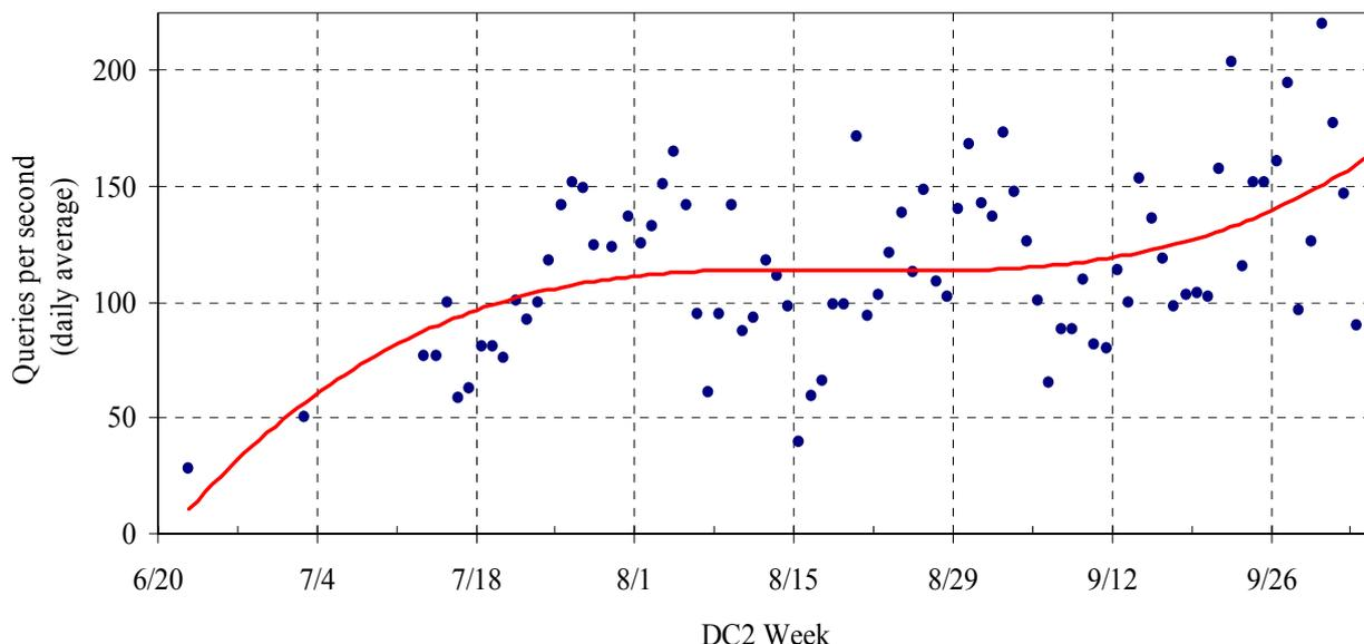
Figure 5: A growing server load from chaotic NOVA database access patterns in ATLAS DC2 production on the Grid.
