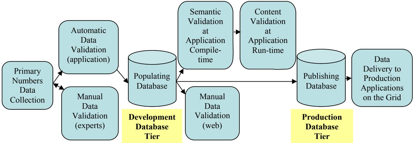
Figure 2: Workflow architecture for capturing, controlling and disseminating ATLAS detector description knowledge. Multiple validation and publishing steps are integral parts of the primary numbers data flow.
