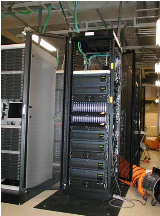
Figure 2: Four file servers with eight 16 300GB IDE RAID systems
