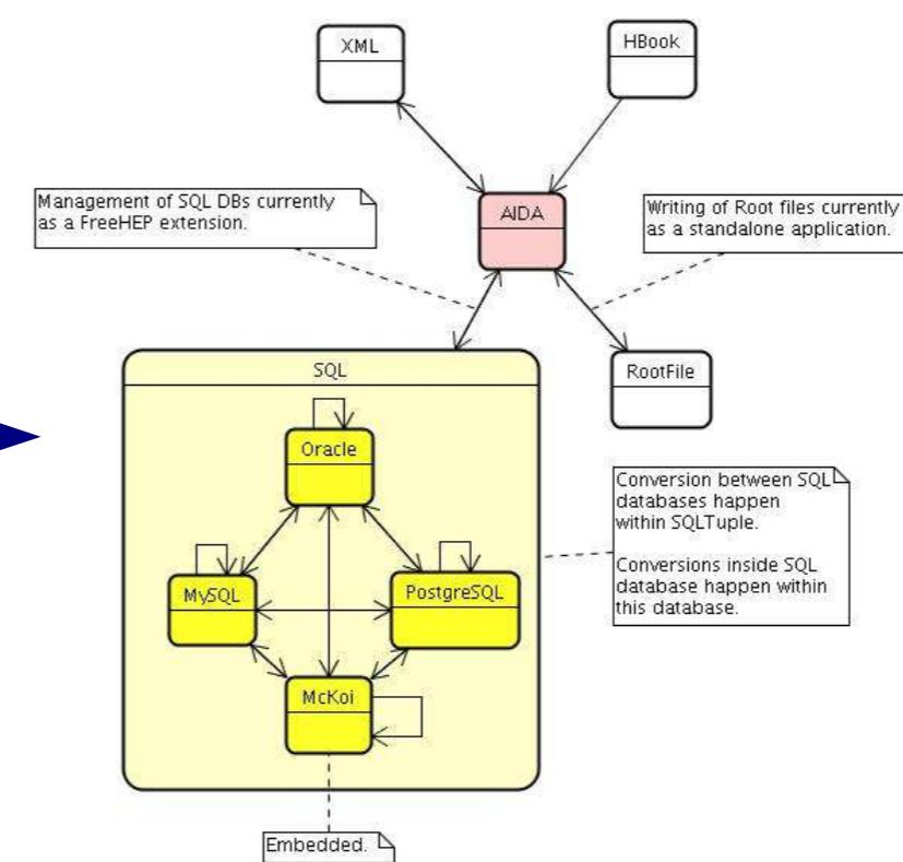
AIDA NTuples can be stored using many different storage technologies (Compressed XML files, Root files, HBook files, several SQL databases).
