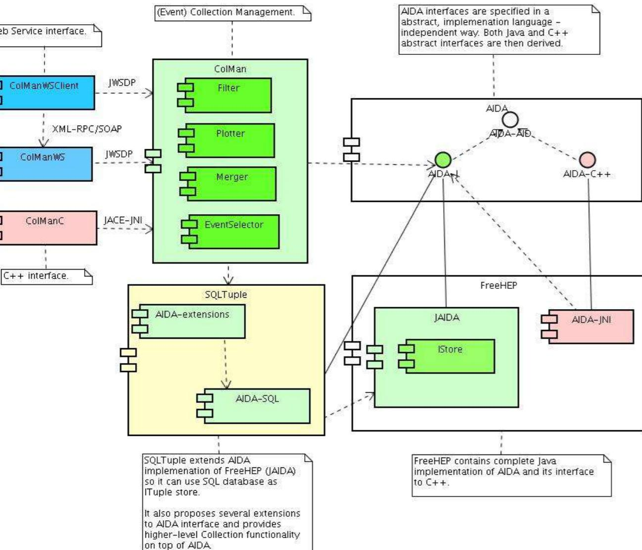
SQLTuple implements AIDA interface as an extension of the FreeHEP JAIDA implementation. ColMan contains several extensions (Filter, Plotter, Merger, EventSelector, Replicator) using AIDA to perform global operations on NTuples (not only SQLTuples). All the functionality is available using standard AIDA interfaces, WebService access and JACE-created C++ proxies.
