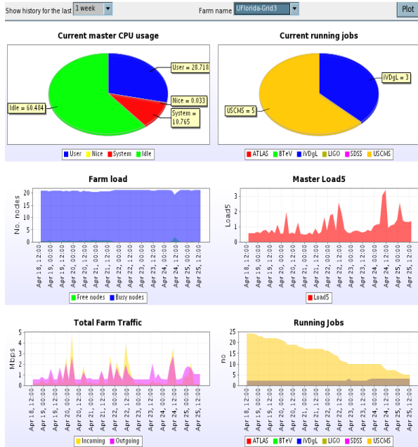
Figure 4. Plots presenting the recent history for the major parameters (jobs running, farm load, total traffic) at UFlorida Grid2003 center.
