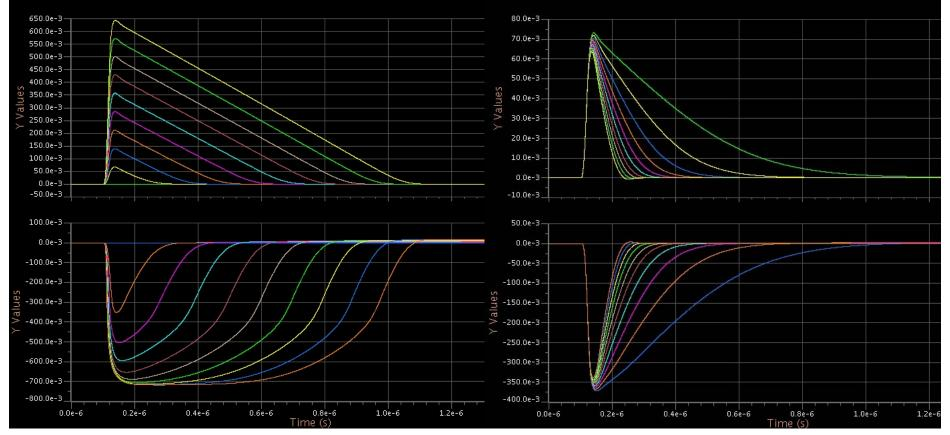
•Left plot is preamp/second stage for charges from 5Ke to 50Ke (20Ke is 500ns TOT). Right plot is for charge of 5Ke and feedback from 2nA to 20nA.
