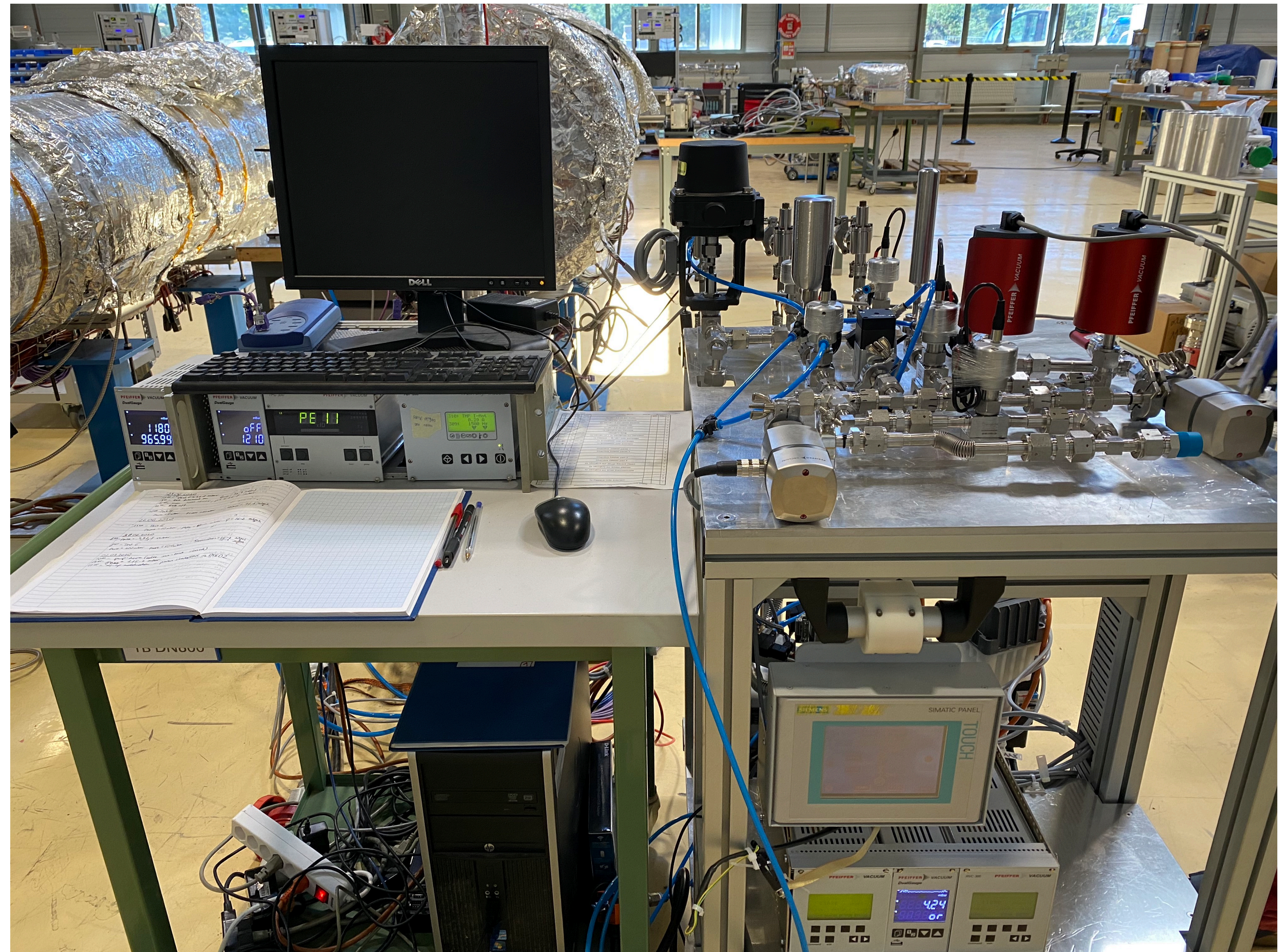
Gas Feed System
