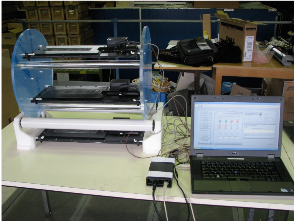
“cosmo-detector” (France) 3 rotating scintillator planes
