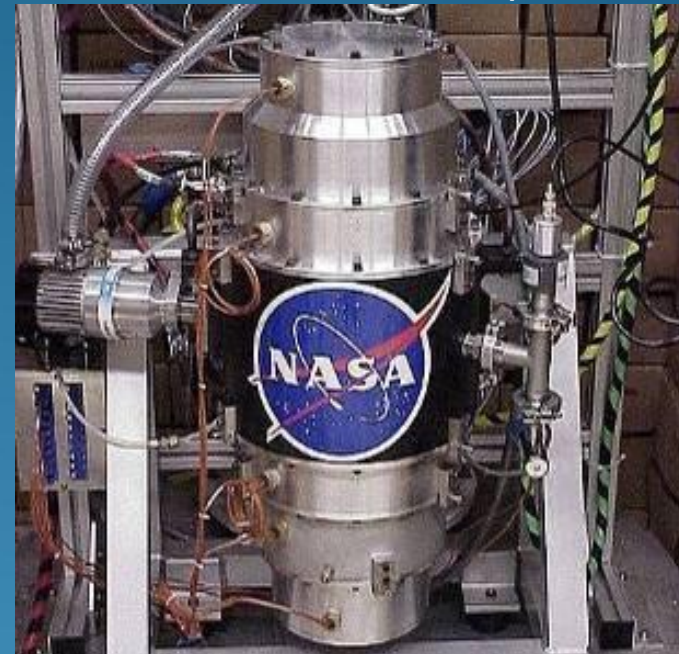
Nasa G2 flywheel: Magnetic bearings, vacuum chamber. Carbon-fiber rotor at 50 000 rpm
