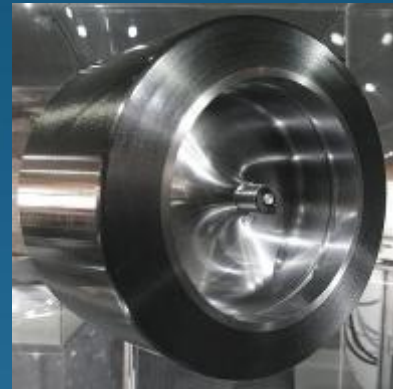
Nasa G2 flywheel: Magnetic bearings, vacuum chamber. Carbon-fiber rotor at 50 000 rpm
