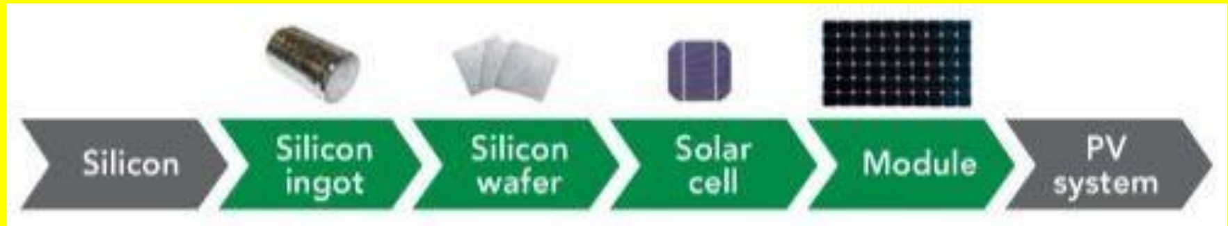
Figure : System build process flow. (Crystalline Silicon)
