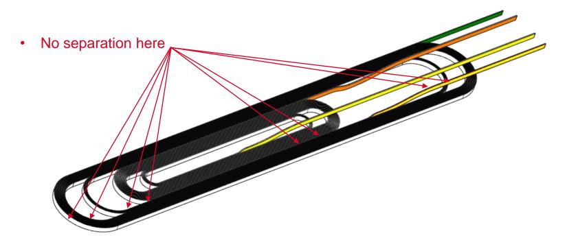
• While keeping the conductor in its safe stresse zone (<200 MPa)
