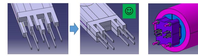
• c) Rods pressure is applied directly to the Horseshoe (mechanical bypass or sliding interfaces)
