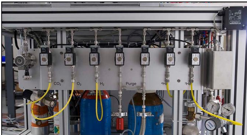
Example: Supernanogan at CNAO (all gas system components included on each IS bench)
