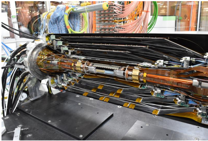
Vertex detector before installation
