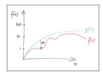
$\Rightarrow$  Accepted x now distributed according to f(x). This algorithm is excessively used in Monte Carlo generators.
