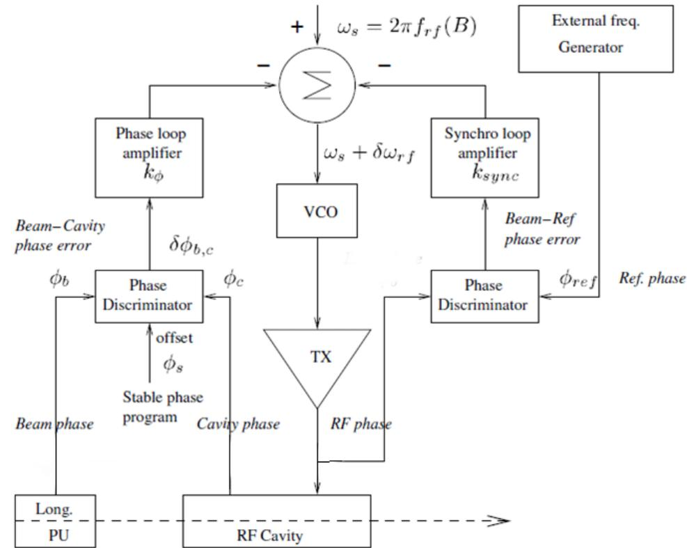
Classic combination for proton and ion synchrotrons: Phase loop and Synchro loop. In the LHC we use a VCXO and the phase loop uses a vector Sum of the eight cavities
