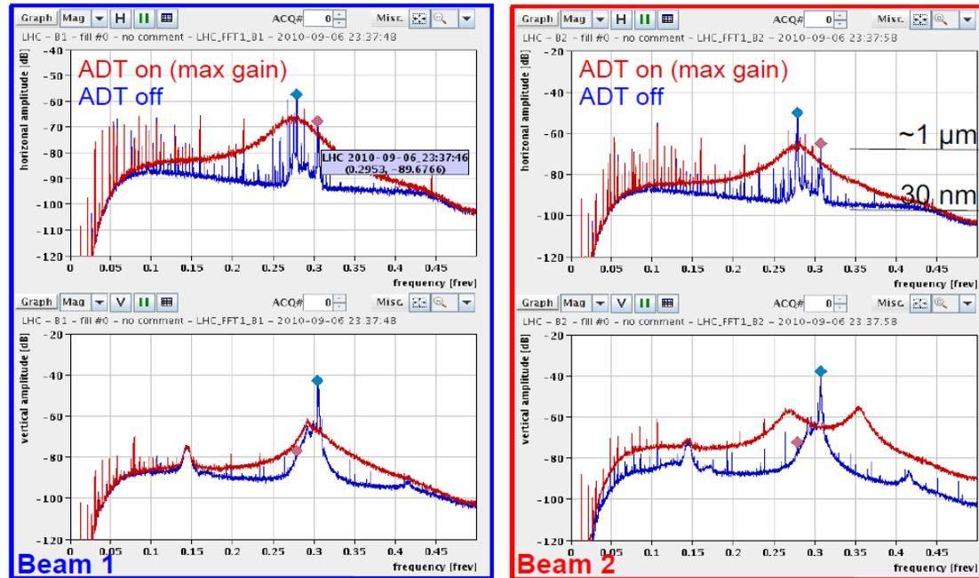
The noise injected by the ADT kickers leads to broadband excitation of the beams that are measured by the Tune system. Outside the betatron band the ADT is virtually open-loop as there is no coherent reaction from the beam.
