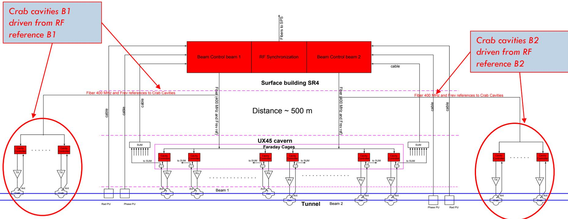
We propose to drive the Crab Cavities from the RF reference (Beam Control, VCXO out)
