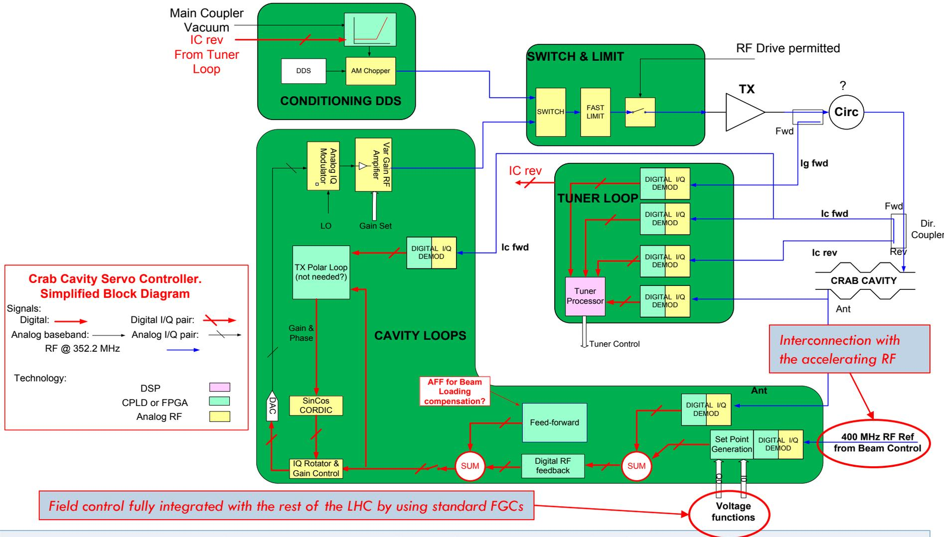
For each Crab Cavity we would have a Cavity Controller similar to the one used on the ACS including:
