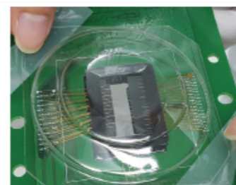
Needles of Probecard 67 needles to contact
