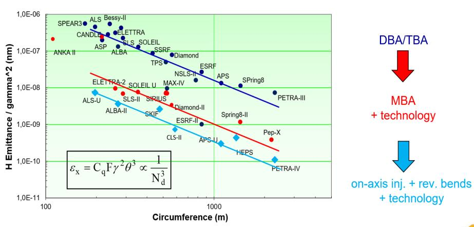
Multibend achromat (MBA) technology underpins the development of diffraction limited light sources
