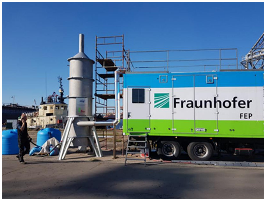
Figure 7. Photo of EBFGT installation at Riga Shipyard. Mobile accelerator unit (right) and wet scrubber (left).
