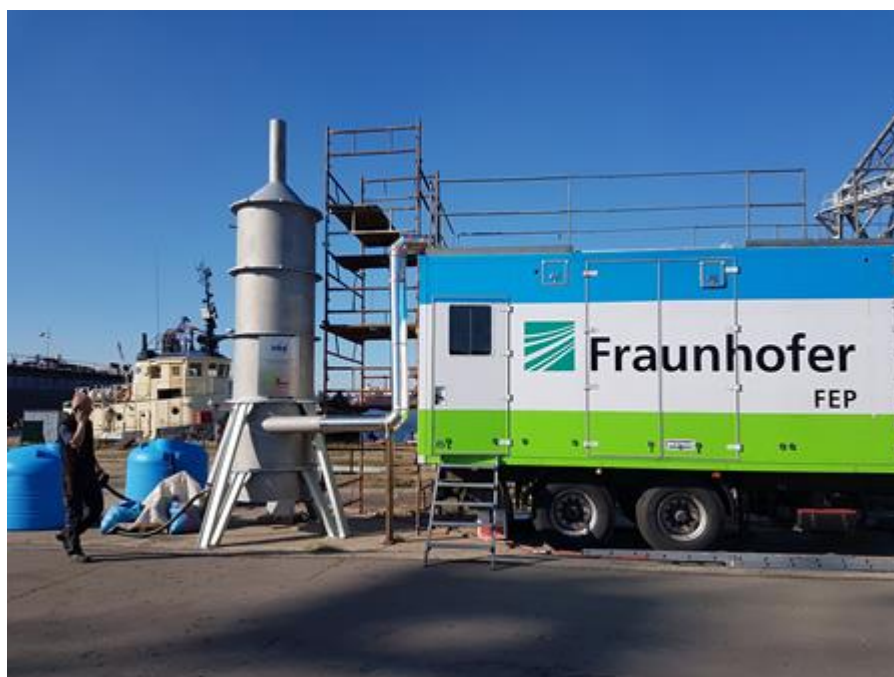
Figure 5. View of trailer hosting FEP accelerator and scrubber connected to the eb system.
