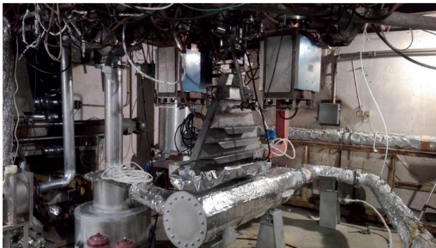
Figure 4. Photo of EBFGT pilot laboratory flow system. Wet scrubber (left) and process vessel (right) under ILU 6 electron accelerator scanning horn.
