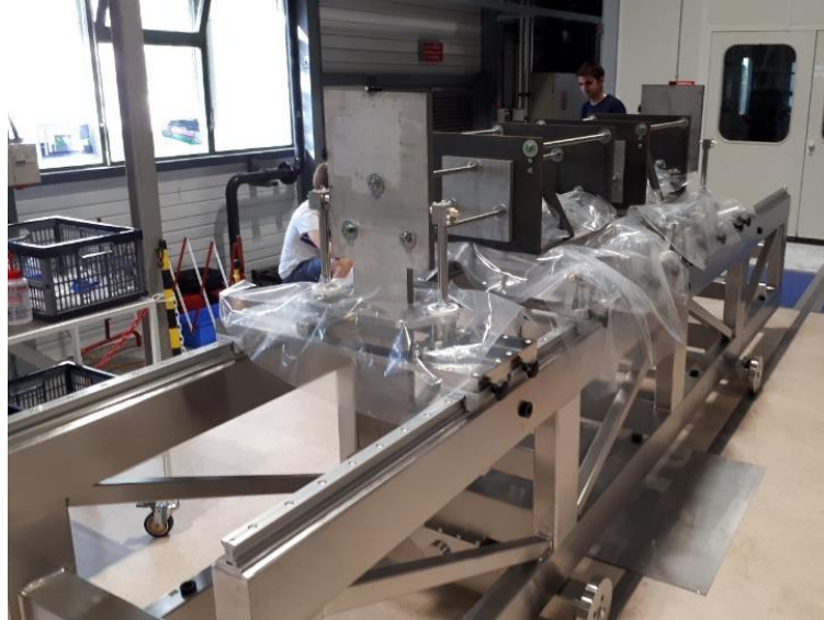
Figure 5 : Control of the trolley rails with loads
