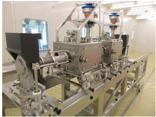
Figure 2 : Trolley for the assembly (with string line assembly)
