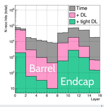
**Loose doublet** selection required to be consistent with the finite beamspot size: σ<sub>z</sub> ~10 mm
