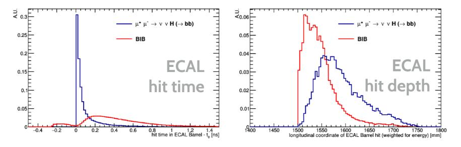
BIB subtraction based on polar-angle, depth and time is under study
