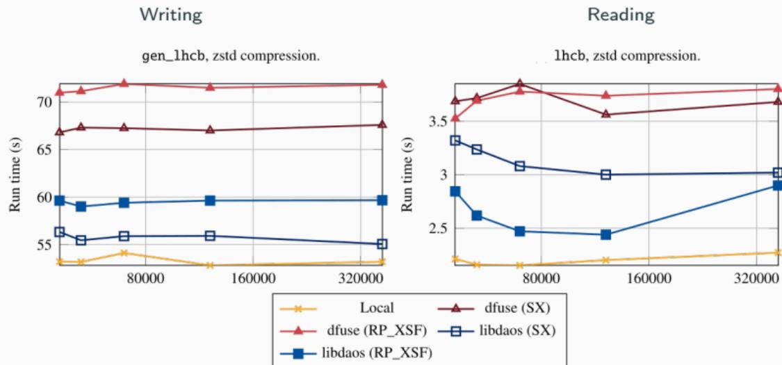
**Figure 3:** RNTuple benchmark from zstd compressed data to histograms on LHCb data (ofi+PSM2). Best raw read throughput: 2.3 GB/s.
