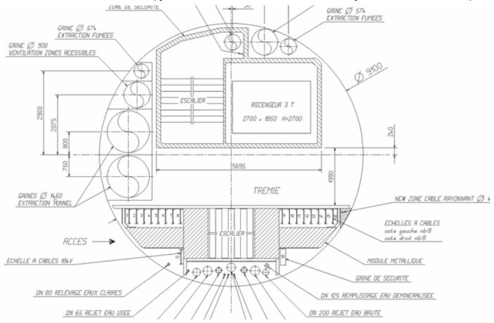
Current design foresees 9.1m diameter shaft (based on HL-LHC shafts). If we could reduce diameter to ~8.5m would save significant money. How much space would be needed for cryo related services (incl. safety).
