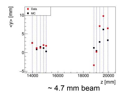
Misalignment generates differences in the amplitude and frequency of TKD oscillations
