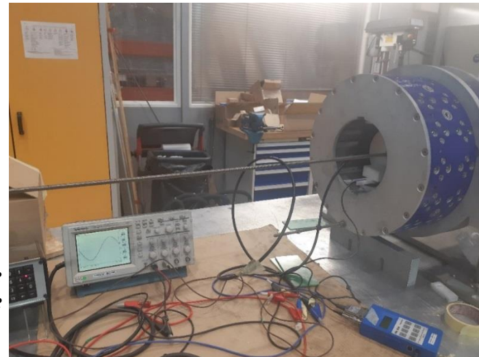
Pictured: system with angular encoder and Hall probe connected to an oscilloscope to check B_r inside the dipole aperture
