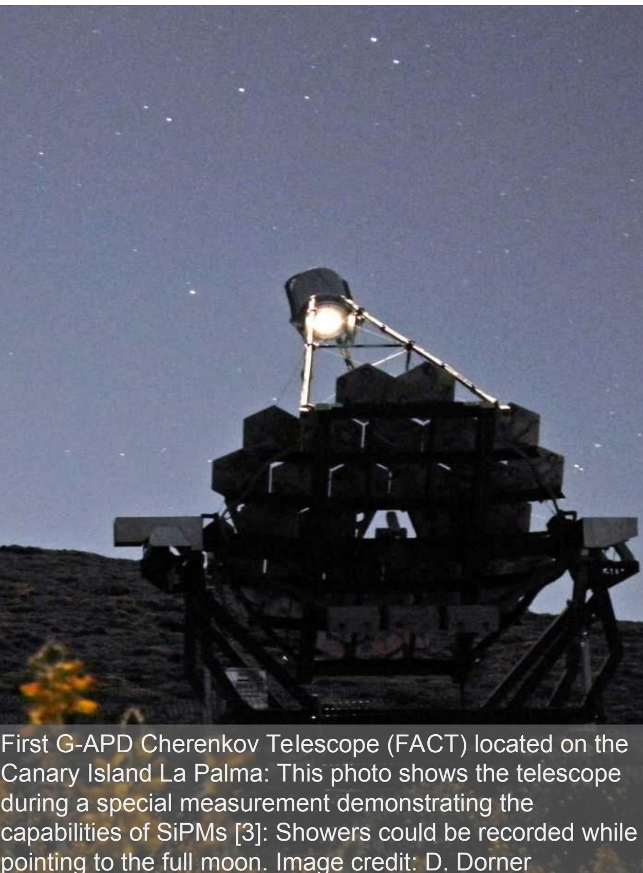
First G-APD Cherenkov Telescope (FACT) located on the Canary Island La Palma: This photo shows the telescope during a special measurement demonstrating the capabilities of SiPMs [3]: Showers could be recorded while pointing to the full moon. Image credit: D. Dorner
