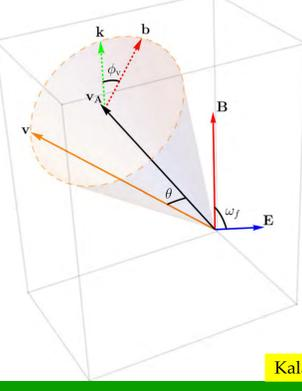
When the particle velocity,  $v$ , is close to  $v_A$ , the particle emits curvature radiation, while for larger  $\theta$  values the particle "gyrates" around  $v_A$  emitting synchrotron radiation.
