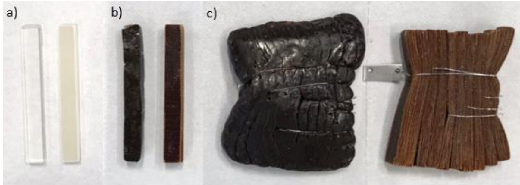
Resin (left) and laminate (right) irradiated at 0 MGy (a), 10 MGy (b), 20 MGy (c)
