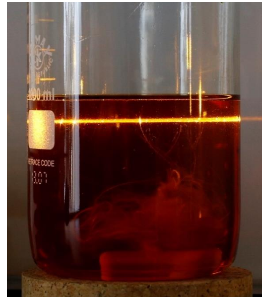
Aramide fiber / DMSO / KOH solution After stirring for 5 days
