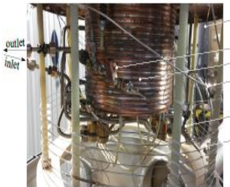
Test bench for JT coefficient measurements at cryogenic temperatures
