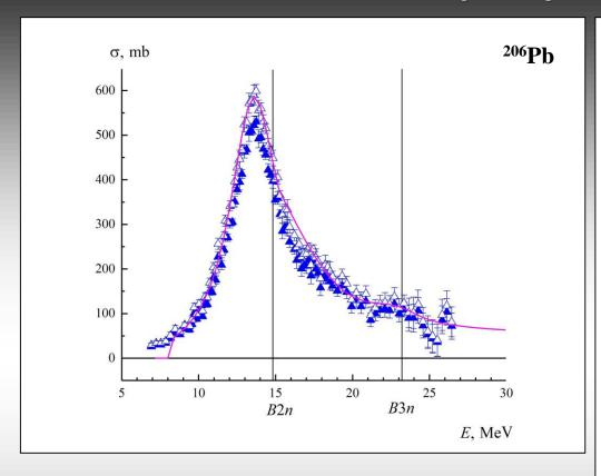
Kcorr =  $\sigma^{\text{theor}}(\gamma, xn)/\sigma^{\text{exp}}(\gamma, xn) = 1927.4/1705.9 = 1.13.$
