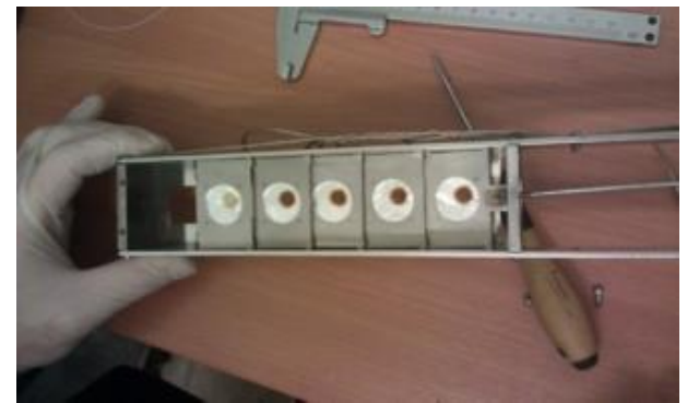
Top: pneumatic actuator with aluminum catcher foils and silicon detectors. Bottom: absorber foils in the position for registration of \alpha -particles
