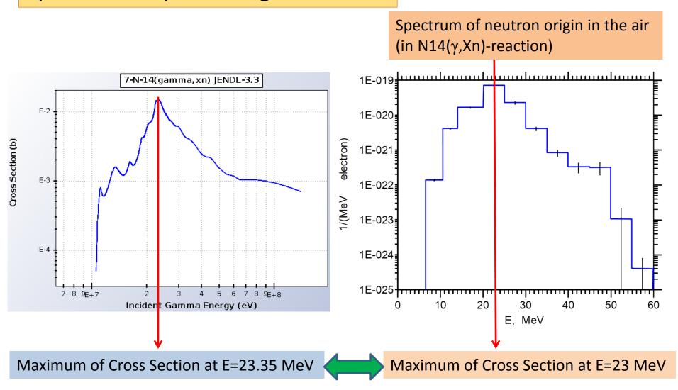
In calculation of the producing neutron spectrum it were taken into account also addition the neutron creation in  $(\gamma,n)$ -reaction 160 ( $E_{threshold} = 15.7$  MeV) and 40Ar ( $E_{threshold} = 10.0$  MeV). It is obtained: 14N, 16O and 40Ar are responsible for 75.3%, 15.7% and 9% of total neutrons yield.
