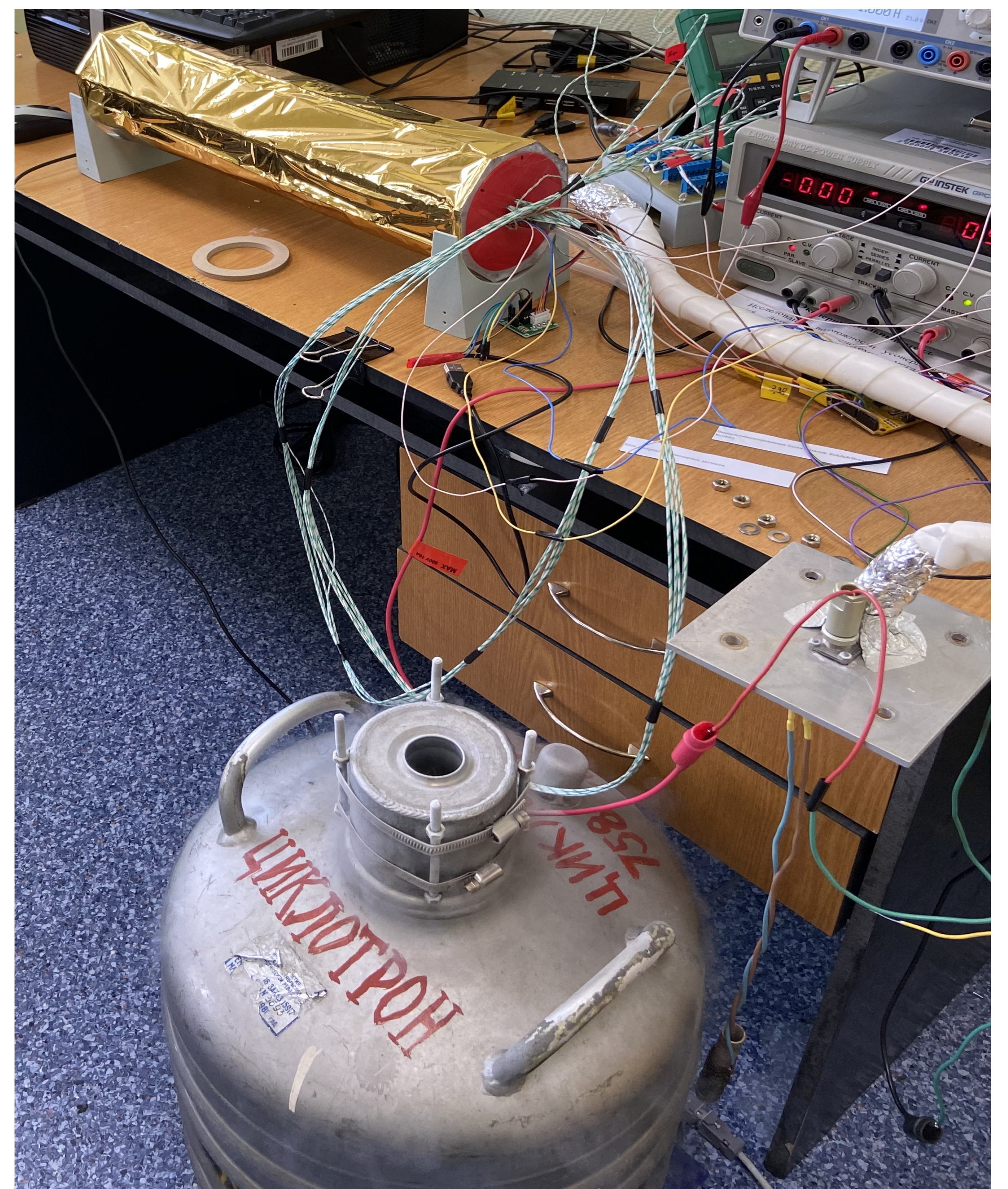
Figure 1. Experimental setup for cooling tests of the mockup of the bent full scale sensor layer.
