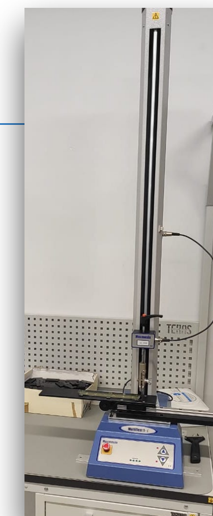
Peel test station
