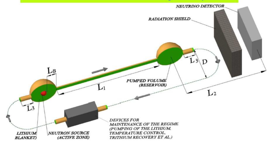
Scheme of the neutrino source with variable spectrum. Lithium in the blanket (activated by neutrons from the source - reactor active zone) is pumped continuously through the delivery channel to the remote volume (reservoir, which is set close to the neutrino detector) and further back to the blanket. The rate of pumping can be smoothly varied by the installation for maintenance of the regime.
