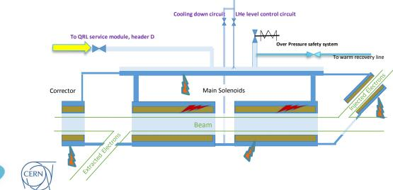
All these possible incidents are addressed by design, if the cryostat is PN 20 and connected to the LHC QRL
