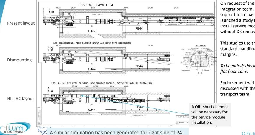
integration team, Cryo support team has launched a study to install service modules without D3 removal.
