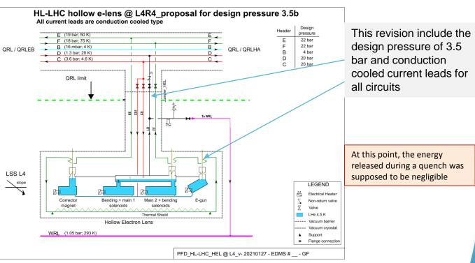
Decision to use conduction cooled current lead is still pending. The gas cooled current lead system is kept in parallel until final choice. A combined solution (120 A conduction cooled & 350 A gas cooled) is also possible.
