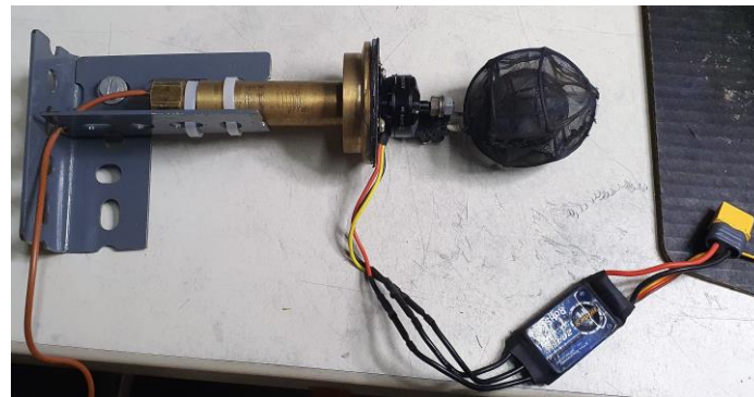
Fig. 15. The motor, ESC, and the spheres
