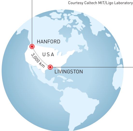
Figure 4. LIGO consists of two gigantic identical interferometers. The gravitational wave first hit the interferometer in Livingston and then passed its twin in Hanford, just over 3,000 km away, 7 milliseconds later. The signals were almost identical, and were a good match with the predicted signal for a gravitational wave. Using the signals, an area in the southern skies could also be identified as the area the waves came from.
